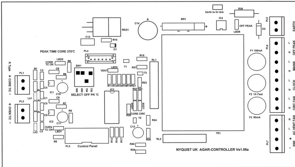
3. Refit Control panel and attach new IDC ribbon cable.
